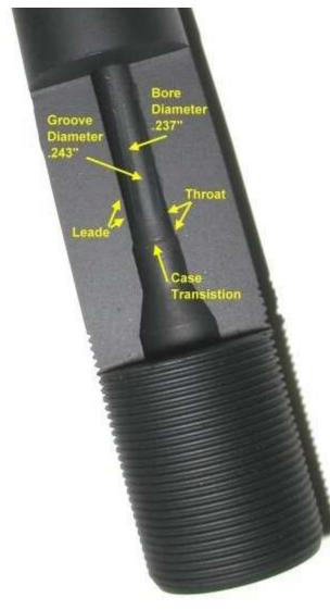
If you run a chamber reamer into a barrel, this will pretty much be the result, without the nifty chamber porting. I didn't want to cut up a good barrel, this is a low buck piece. I clamped it down in a milling machine and lobbed away until I had this cutaway. I think I learned a lesson about rough milling versus finish milling, and I learned that I can't increase the amount of material removed with each pass, just because I'm bored.
