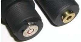
breech is closed. Chambers of exacting dimensions are cut into barrels with reamers.
