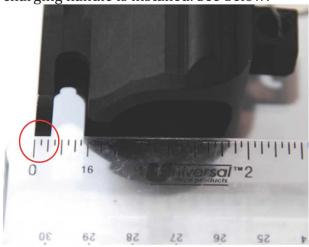
The older "High Profile" upper receiver has a **3/16"** wide top portion where the charging handle is installed. See below:
