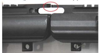
The new "Low Profile" upper receiver has a 1/8" wide top portion where the charging handle is installed. See below:
