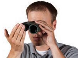
**2. Adjust the diopter** – Start by closing your left eye or covering the left objective lens with your hand. Look through your right eye and adjust the diopter ring (generally found on the right eyepiece) until the object is in focus. Make note of this diopter setting in case you need to set it again. From this point on, you will only need to use the center focus wheel.
