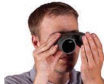
**✓ TIP Locking Diopters** – Some models feature a diopter that locks the settings. If the diopter locks, lift the diopter ring (or follow manufacturer instructions) to unlock. Then, looking through your right eye, adjust the diopter so that the object is in focus. Make note of this diopter setting in case you need to set it again. Push the diopter ring down to lock—from this point on, you will only need to use the center focus wheel.
