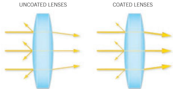
☑ **TIP** The application of more coatings results in an increase of light transmission, resolution, contrast, and color fidelity.
