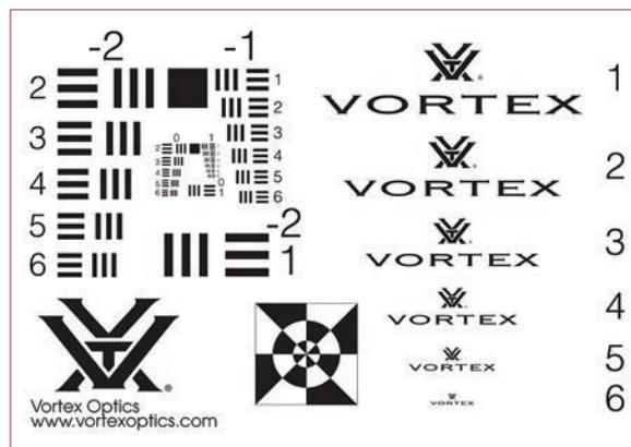
**TIP** Use a resolution chart to determine how well a binocular, spotting scope, or riflescope can resolve fine details.
