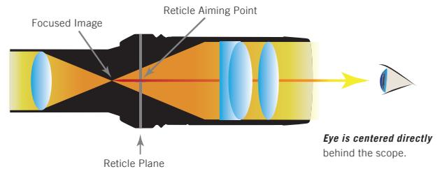
**Tip** Correctly focus the target image so it falls on the same optical plane as the reticle within the riflescope.
