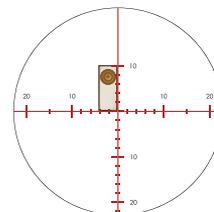
**TIP** You can substitute 100 for 95.5 for faster calculating, but this will produce a five percent over-estimation error of the yardage distance.
