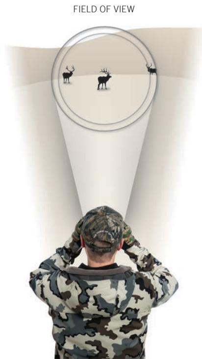
A wide field of view has advantages when following fast-moving action or scanning dense habitats. When comparing optics with the same size objective lenses, higher magnifications will generally have a narrower field of view.
