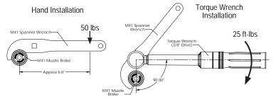
**IMPORTANT:** After installation is completed, it is imperative to check the alignment of the muzzle brake bore with the barrel bore to verify appropriate bullet clearance. This should be checked visually and with a tight fitting bore alignment rod inserted through barrel and muzzle brake to verify a bullet will not impact.
